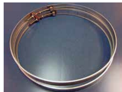
Cleaned Stainless Steel Bands Prior to Testing
