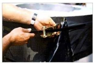
2. Insert the loose strap and through slot in the take-up shaft. Push down and up on handle to apply tension. Once proper tension has been achieved push handle down to lock into position.
